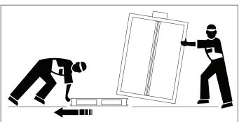
After removing the pallet, lower the cabinet slowly and without jolts to avoid damaging it.
