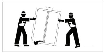
After installing the cabinet, remove the protections for transport present along the door joints.
