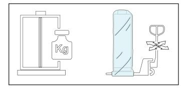
Use a pallet truck to move the cabinet, which must be placed vertically and be secured and protected against slipping up to its final installation site.
